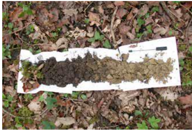
Figure 3 A soil profile derived with a Dutch soil auger. Samples are taken from the same core site and laid out in sequence (i.e. topsoil above subsoil above parent material) to ascertain the soil type.
