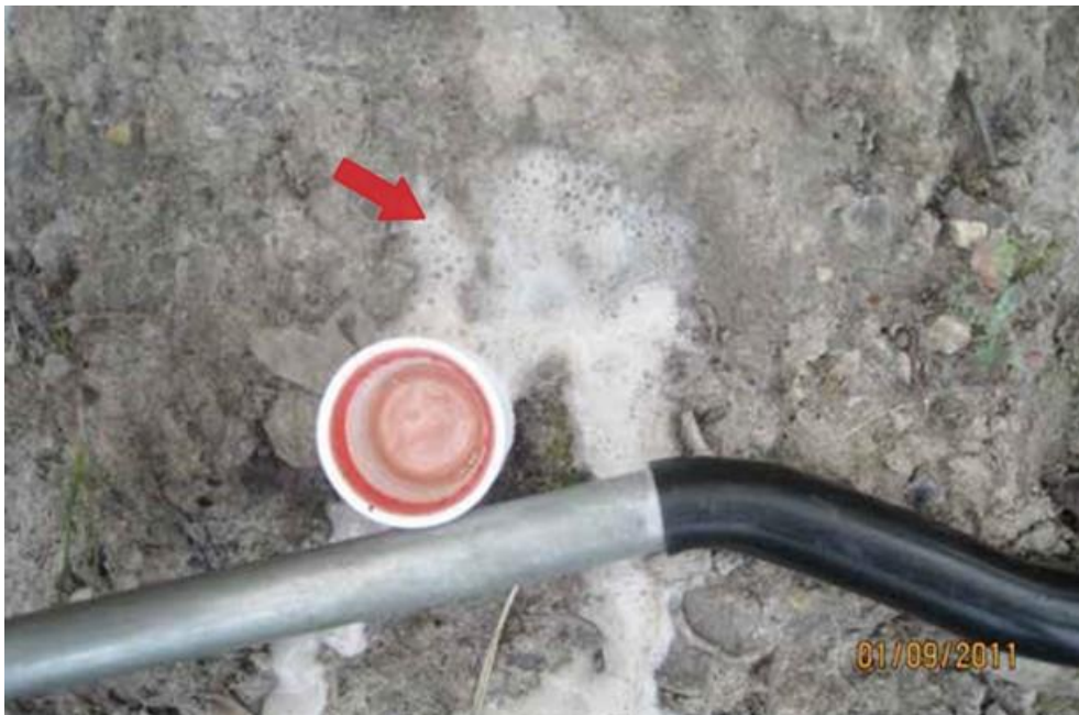
Photo 1 Soil core displaying vigorous effervescence with dilute (10%) hydrochloric acid.
