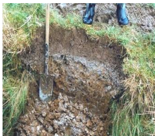
A very poorly drained 'dauby' gley soil profile with a clay-rich topsoil approx. 30 cm deep, which overlies a saturated & mottled, blue-grey & red-brown subsoil. The subsoil overlies a very compact parent material derived from glacial till.
